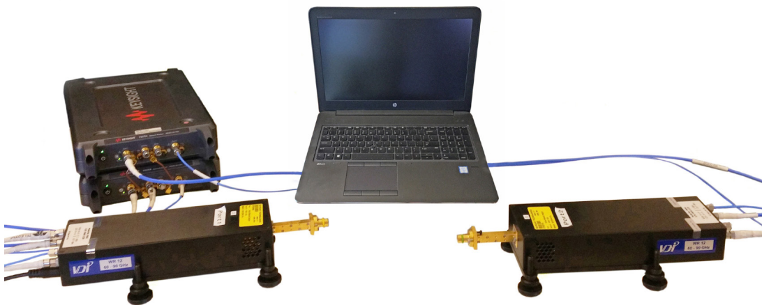
Figure 5. P9375A Streamline USB VNA based E-band VNA setup
